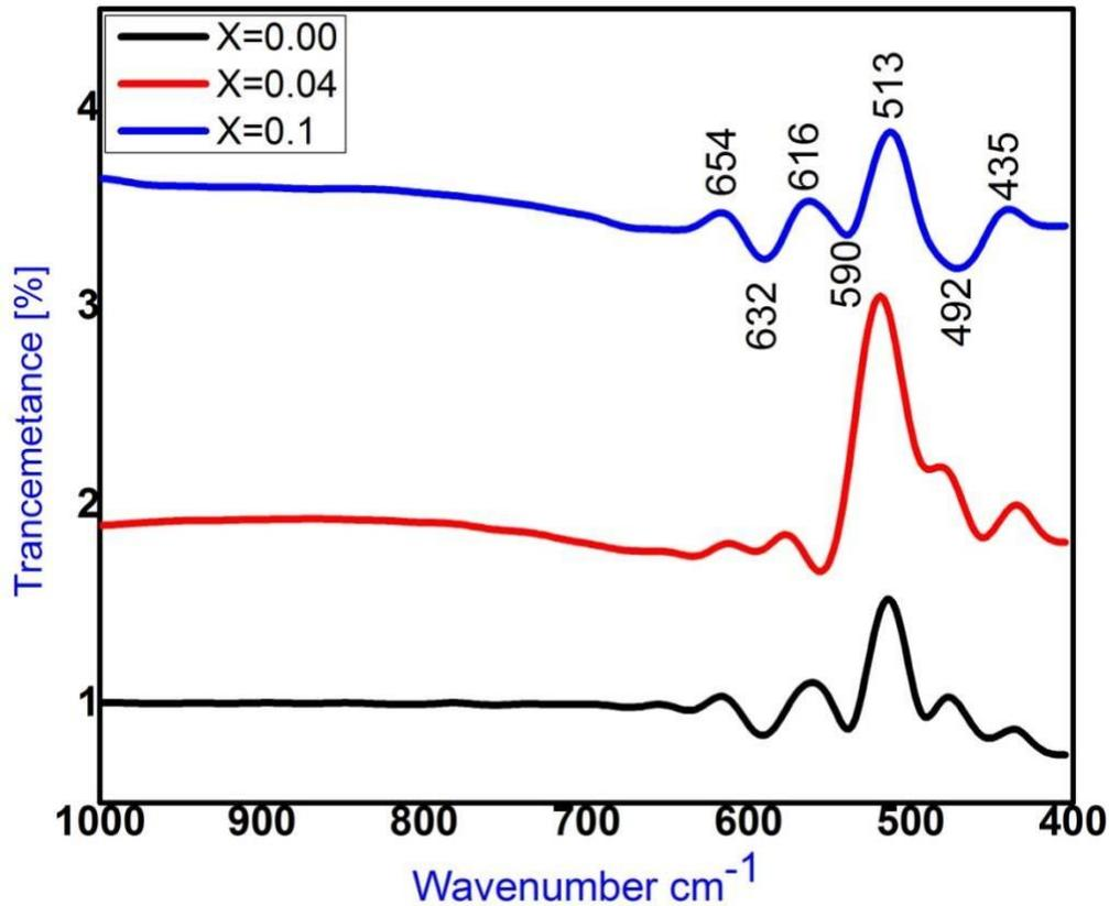
**Figure 1:** The FTIR of  $\text{Ca}_{1-x}\text{Al}_x\text{CO}_2\text{Fe}_{16}\text{O}_{22}$ , ( $x = 0.00 - 0.10$ ) annealed at  $900^\circ\text{C}$
