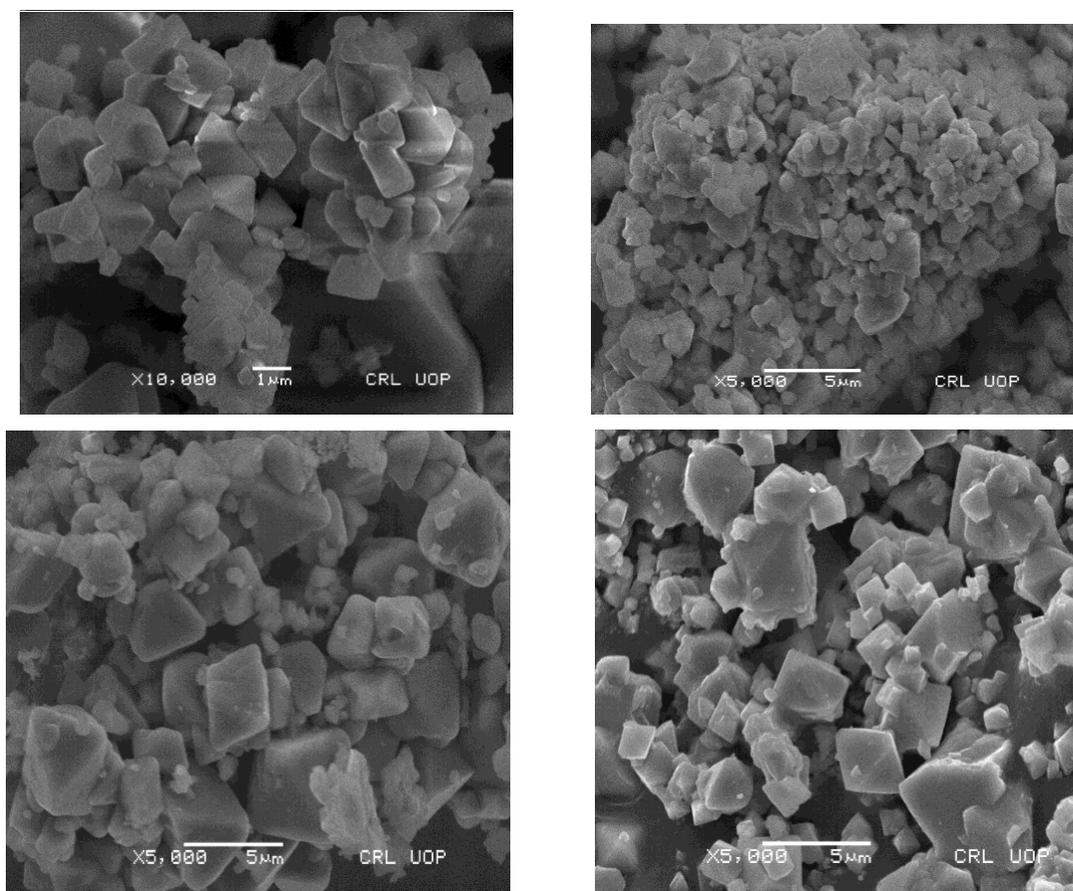
**Fig 3:** SEM images of  $\text{Ca}_{1-x}\text{Al}_x\text{CO}_2\text{Fe}_{16}\text{O}_{22}$ , ( $x = 0.08 - 0.10$ ) at  $1\mu\text{m}$  to  $10\mu\text{m}$  scale.
