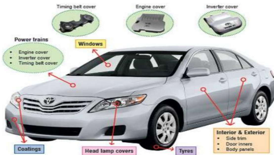
Fig. 13: Components of the car in which polymer nanocomposite are used
